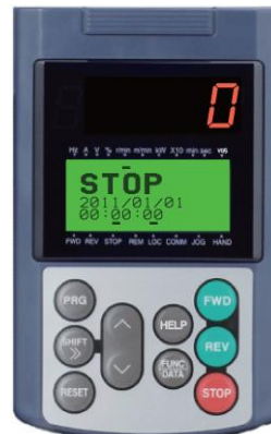
Figure 4.2-1 Display of the LED Monitor at Power-on
